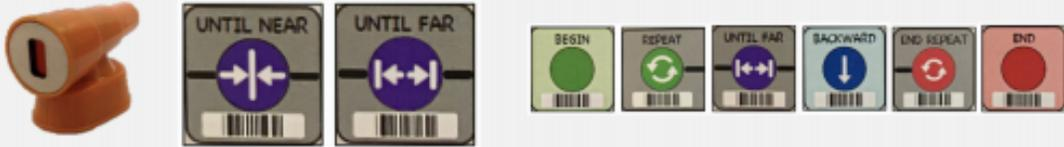
The image shows a KIBO robot head on the left. Next to it are two parameter blocks: 'UNTIL NEAR' with a double-headed arrow icon and 'UNTIL FAR' with a double-headed arrow and a vertical line icon. To the right is a sequence of programming blocks: 'BEGIN' (green circle), 'REPEAT' (green circle with arrow), 'UNTIL FAR' (blue double-headed arrow icon), 'BACKWARD' (blue downward arrow icon), 'END REPEAT' (red circle with arrow), and 'END' (red circle).
